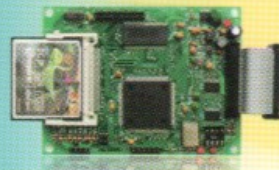
แผงวงจร EVM Embedded Voice Management Card
